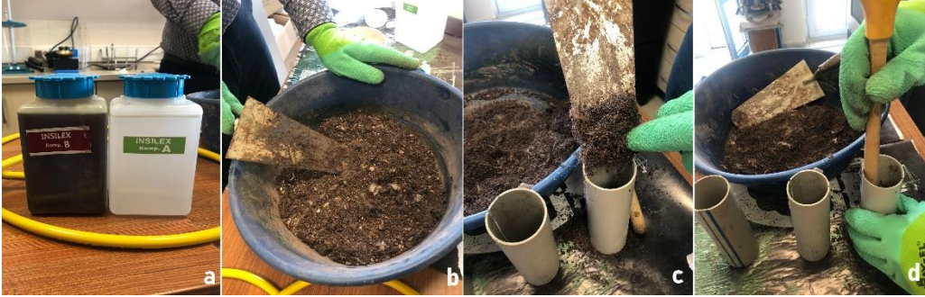
Figure 3. a) Components of the resin, b) specimen mixing, c and d) specimen molding
