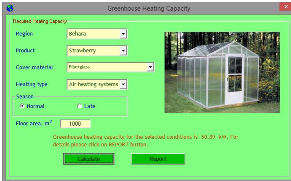
Figure 4. The calculation of the heating capacity required for a greenhouse for strawberries in the Behara region
