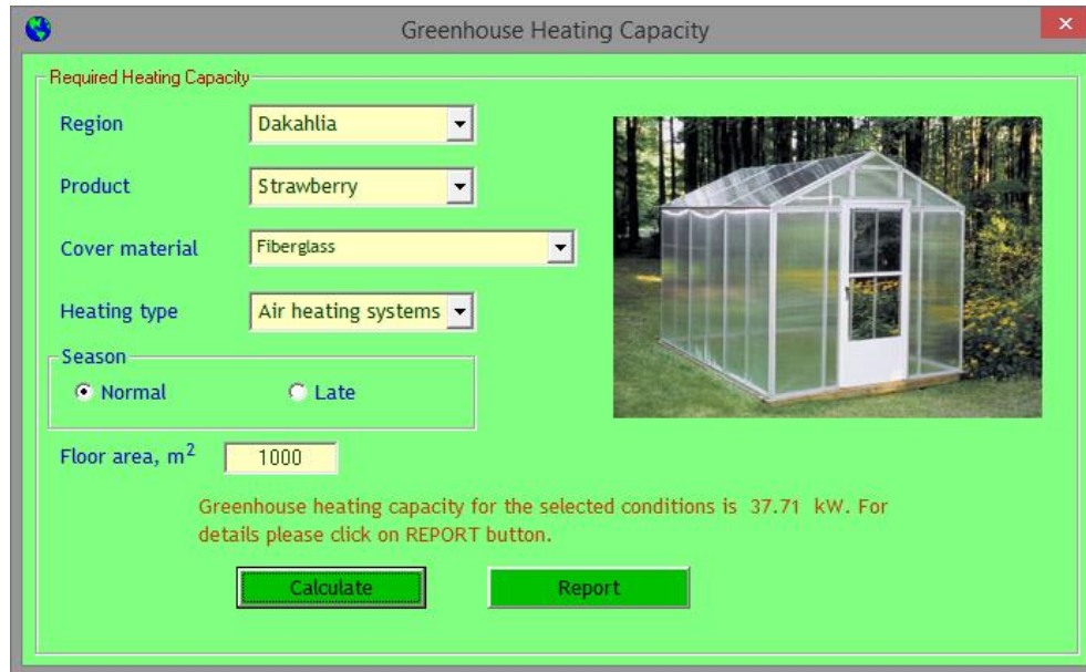
Figure 2. The calculation of the heating capacity required for a 1000 m 2 fiberglass greenhouse for strawberries in the Dakahlia region
