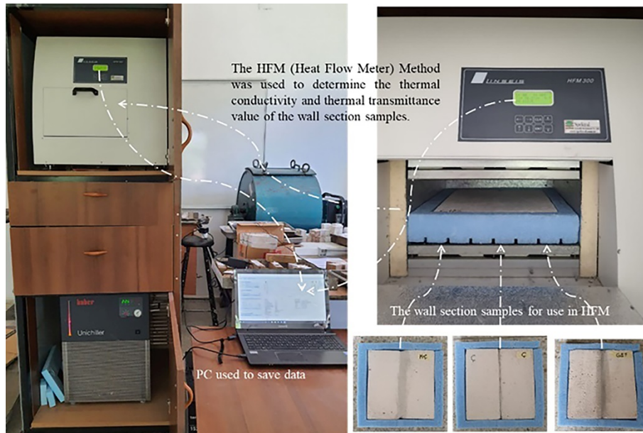
Figure 1. Heat flow meter method (coded HFM 300)
