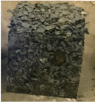
Figure 2: Concrete cube made using 100% replacement of natural aggregates with polypropylene (PP) plastic waste (WP-Concrete).
