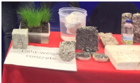
Figure 3: An exhibition of the wide variety of concrete containing waste plastics, showcasing growing of grass and floating of the concrete in water (concrete in the plastic container), among other unique characteristics.
