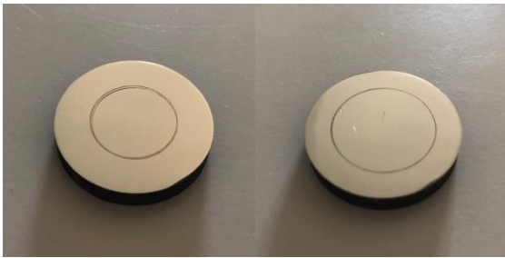
Figure 21. Wear marks on the D2 steel sample after testing with the (a): manufactured tribometer, (b): CSM tribometer
