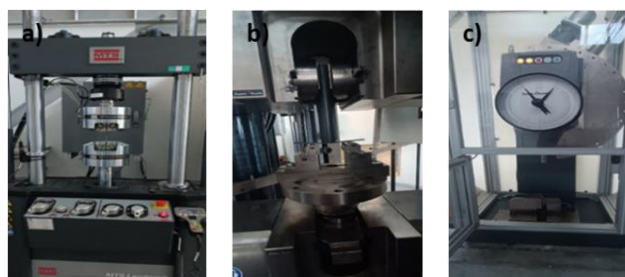
Figure 2. a) A Tensile testing machine, b) a Flexural bending test machine, and c) an impact testing machine.
