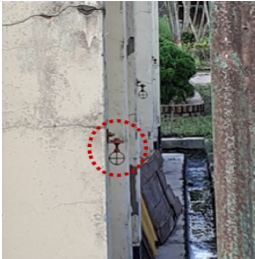
Fig. 5. (a) Prism layout plan, (b) Prism installed on the adjacent school building and (c) Prism installed on the capping beam
