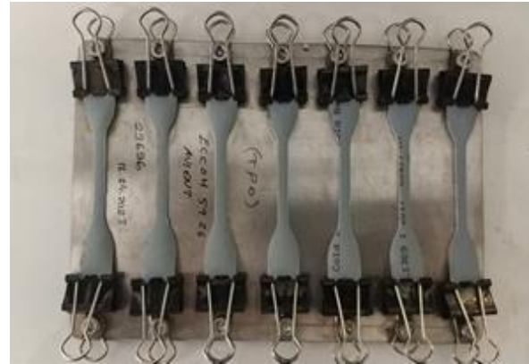
Figure 3. The thermoplastic polyolefin dumb-bell pieces prepared.
