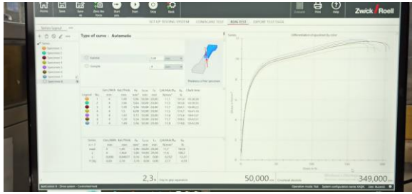
Figure 8. The screen of the Zwick/Roell machine interface program showing the test results of the thermoplastic polyolefin dumb-bell pieces after the tensile strength test.
