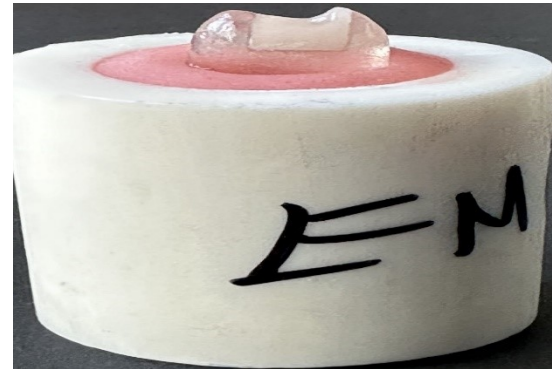
Figure 3: Sample embedded in acrylic resin
