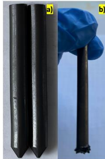
Figure 3. Image of (a) anode and cathode electrodes before and (b) cathode electrodes after electrolytic exfoliation reaction
