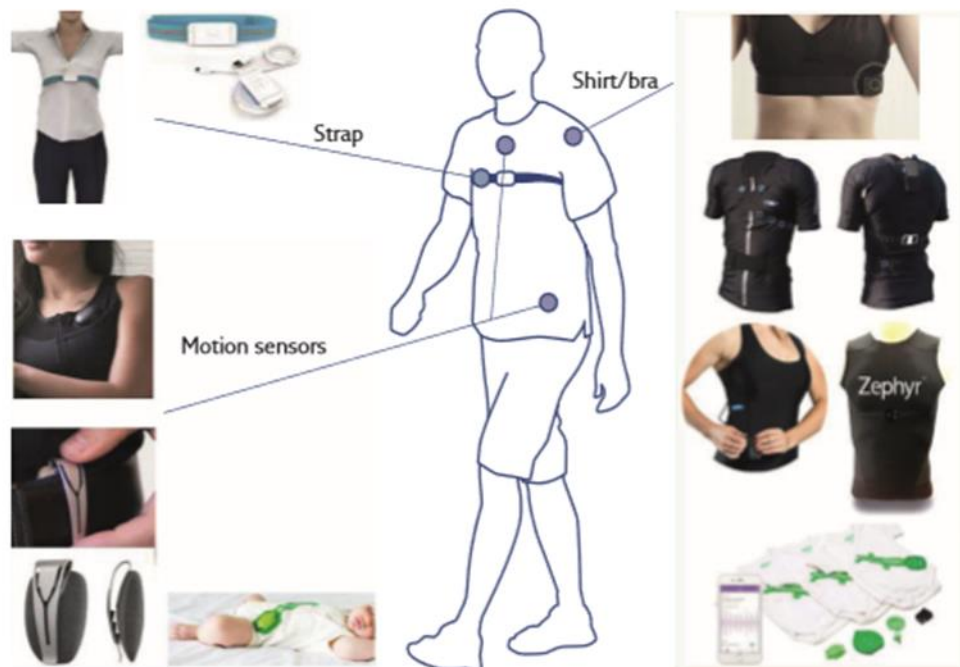
Figure 1. Location of various wearable devices on the body that can estimate ventilation from chest surface movement [8].
