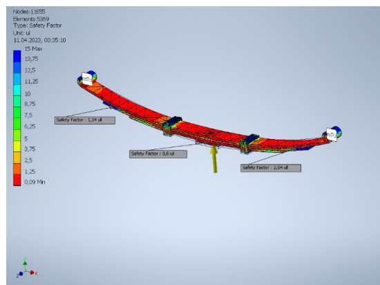
Figure 6. Von Mises stress, displacement, safety factor results of steel alloy material under 100000 N load
