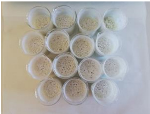
Figure 1. hBN coated PA 66/GF30 granules.
