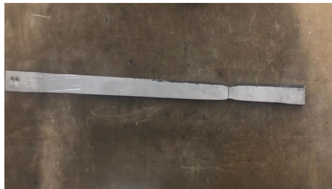
Figure 6. A broken tensile test sample
