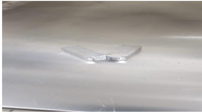
Figure 7. A broken impact test sample
