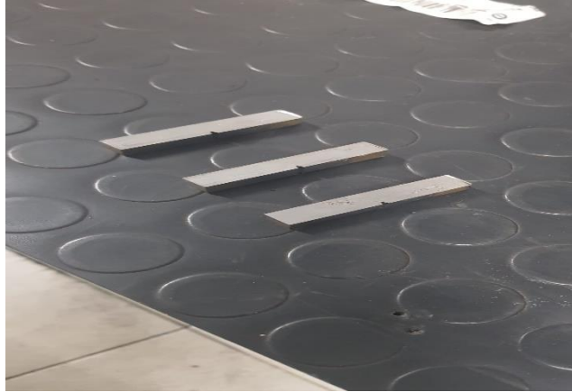
Figure 2. Sample prepared for the impact test
