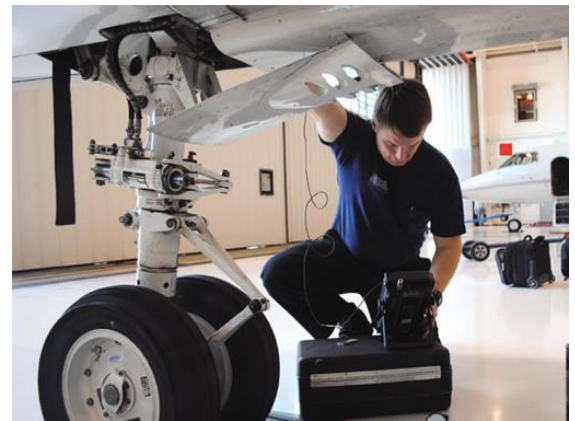
Fig. 5. Magnetic testing of landing gear components [18]
