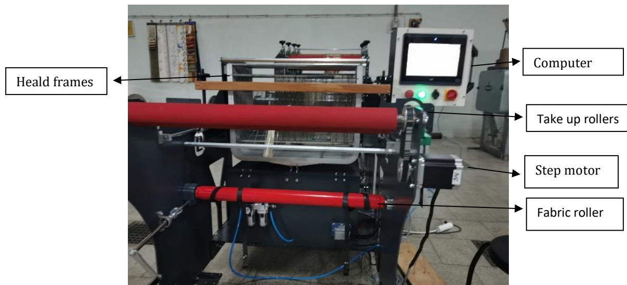
Figure 1. Front view of the sample dobby weaving machine
