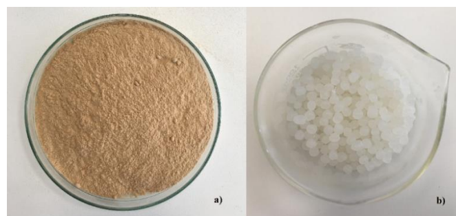
Figure 1. Wood flour (a) and PLA (b)
