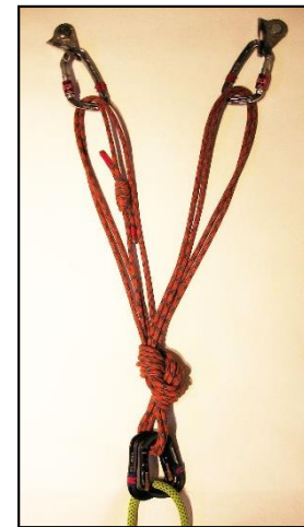
Figure 5. A cordelette tied with a double cord. Rope attached to opposed HMS carabiners and multi-strand Figure Eight Loop. (Figure 4 labels apply to this image.)
