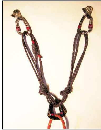
Figure 7. Quad with paired carabiners using a double cord. Rope attached to opposed HMS carabiners and cord segments isolated with two multi-strand Overhand Loops. (Figure 6 labels apply to this image as well.)
