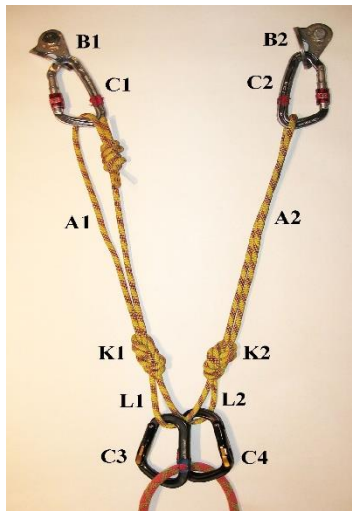
Figure 8. Quad with separated carabiners using a single cord. Rope attached to separated HMS carabiners and cord segments isolated with two Overhand Loops.
