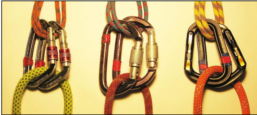
Figure 1. Carabiner orientations, from left to right: unsafe parallel D carabiners because they open on the same side in the same direction; reversed D carabiners, which open in opposite directions; opposed HMS carabiners, which open on opposite sides.
