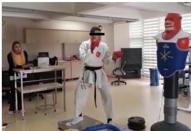
Picture 1. Repetitive kick force and duration test (Source: Captured by authors.)
