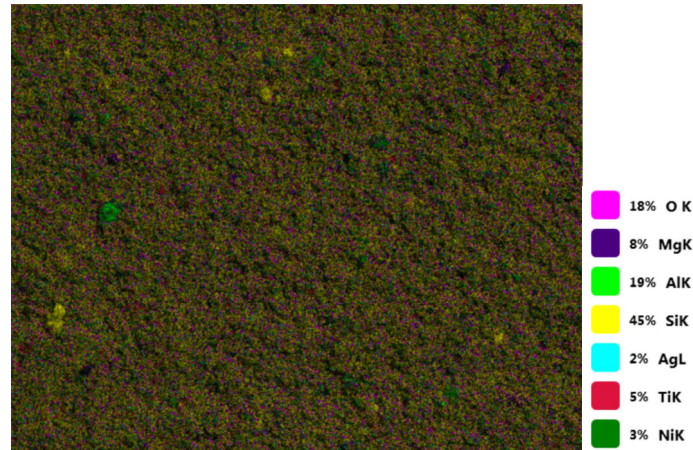
Figure 7. SEM mapping result of Ag-Ni-TiO 2 /Cordierite catalyst
