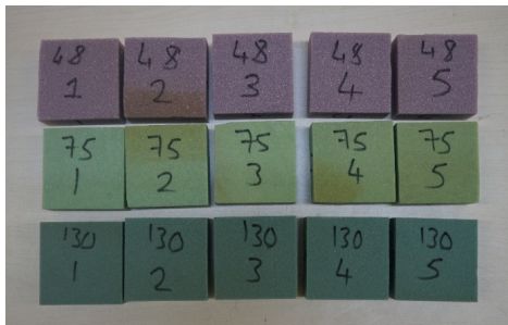
Figure 2. PVC foam specimens prepared for compression testing
