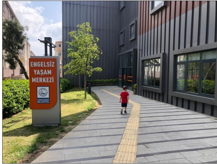
Figure 6. Building entrance accessible for users and yellow wayfinding floor sign (image by authors)
