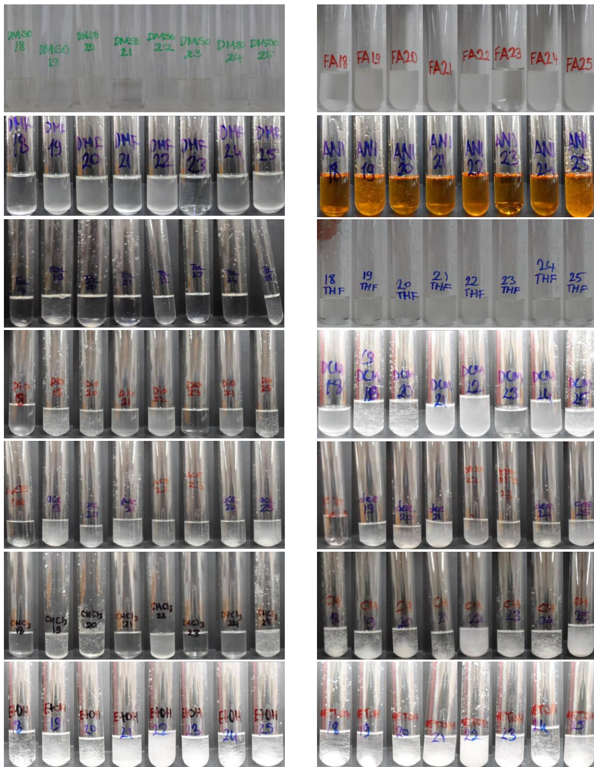
Figure 1. The photographs showing the chemical resistance of cellulose acetate samples, synthesised under the solvent effect of ethyl lactate, in some solvents (Abbreviations, DMSO: Dimethyl sulfoxide, FA: Formic acid, DMF: Dimethylformamide, ANI: Anillin, TOL: Toluene, THF: Tetrahydrofuran, DIO: Dioxane, DCM: Dichloromethane, ACE: Acetone, DEE: Diethyl ether, CHCl 3 : Chloroform, CH: Cyclohexane, EtOH: Ethyl alcohol, MetOH: Methyl alcohol). The numbers in the pictures, 18: 1EL20S010, 19: 1EL20S025, 20: 1EL20S050, 21: 1EL20S100, 22: 1EL40S010, 23: 1EL40S025, 24: 1EL40S050, 25: 1EL40S100).
