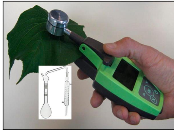
Figure 1. Dualex+ 4 Scientific (FORCE-A, Orsay, France) cihazı (Cerovic et al., 2015)
