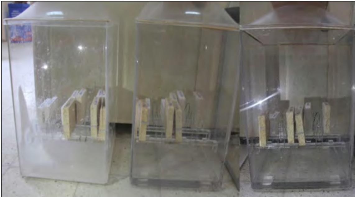
Figure 9- Image of the test for the determination of resistance to ageing by SO 2 in a humid environment.
