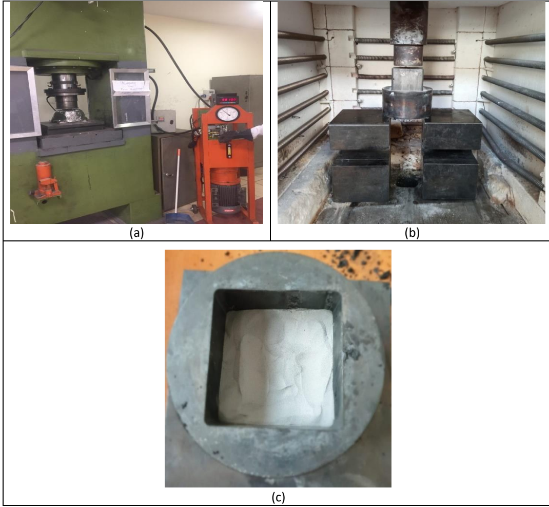
Figure 4. (a) Pressing, (b) sintering and (c) final product ((a)Presleme, (b) Sinterleme ve (c) nihai ürün)
