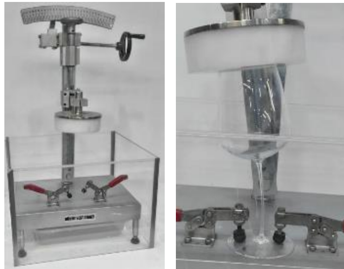
Figure 11. Bend Test apparatus.
