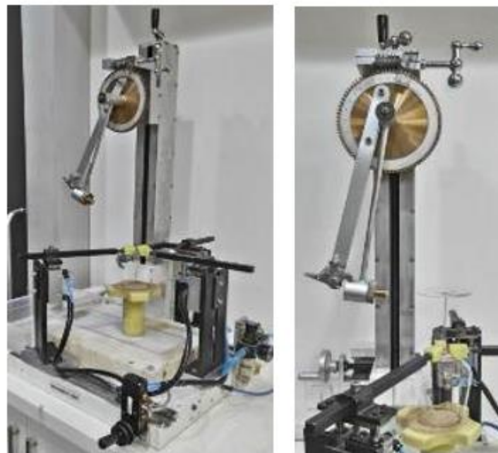
Figure 9. The tool used to test the impact resistance of glass samples taken from the base.
