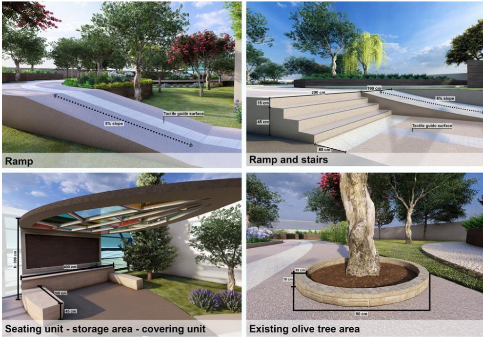
Figure 7. Seating Unit-Storage Area-Covering Unit Existing Olive Trees and Their Surroundings Detail and Dimension Detail
