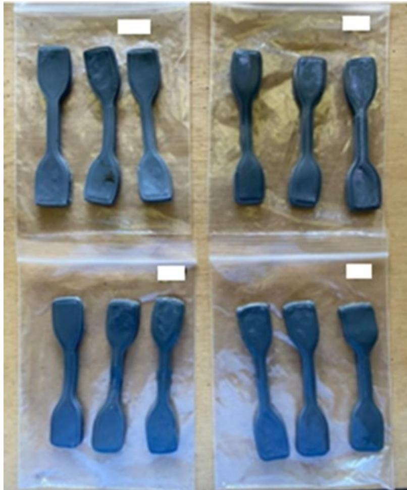
Figure 5: Samples of specimens after annealing process at variuos temperatures and times: (a) 20 min, (b) 40 min, (c) 60 min.
