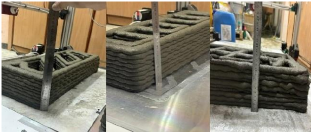
Figure 6. Fresh State Height Measurement
