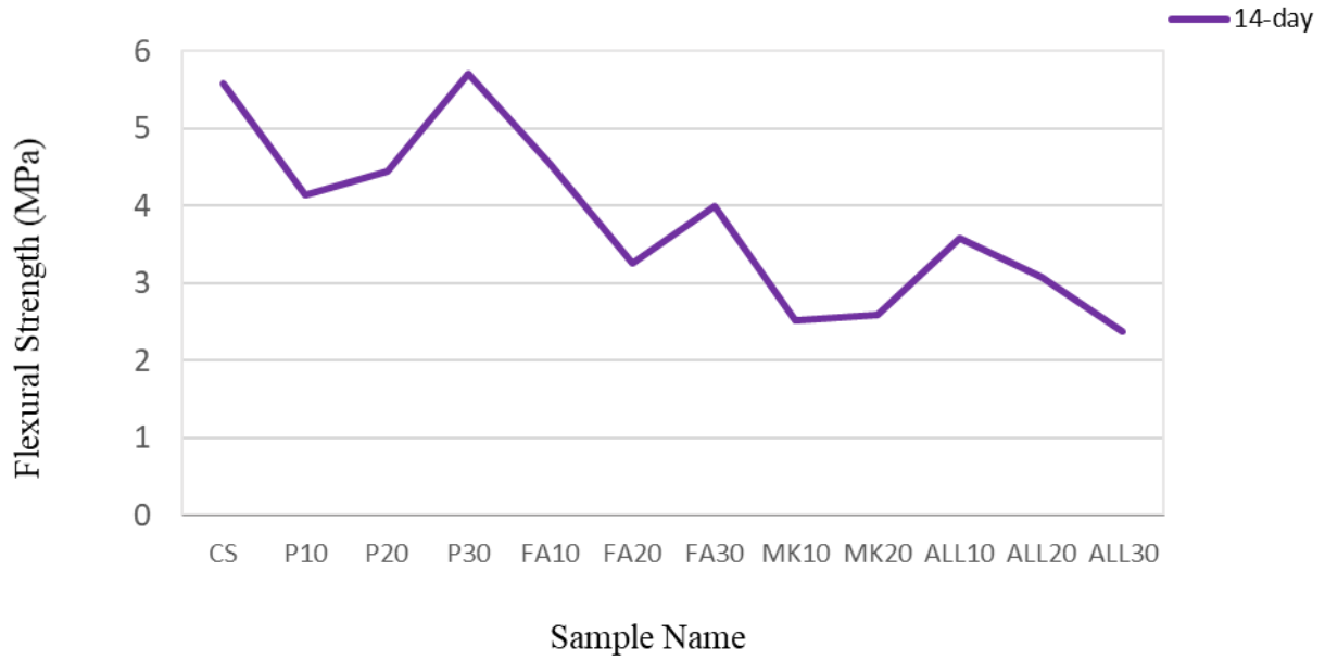
Figure 4. Flexural strength of the composite mortar mixtures
