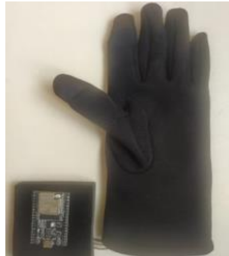
Figure 8. Glove that can measure real-time temperature
