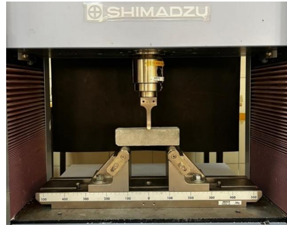
Figure 3. Three-point flexural test
