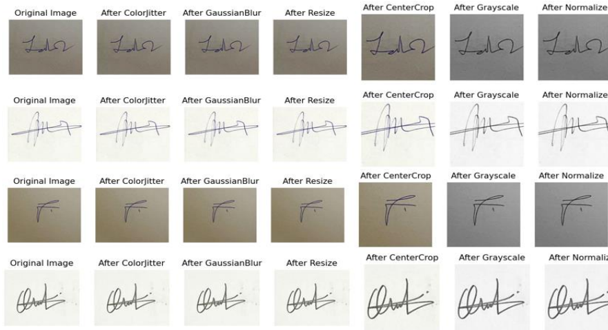
Figure 3. Preprocessing Steps Applied to Several Different Signature Samples from the Dataset
