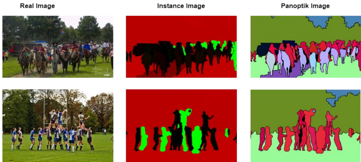
Figure 4. Instance segmentation and panoptic segmentation results for the COCO dataset
