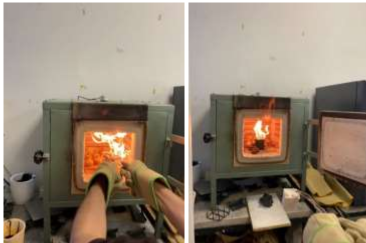
Figure 8. Placing the ceramic pots in the kiln.
