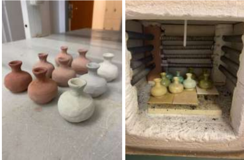
Figure 7. a) Glazed forms before firing. b) Placement in the enamel kiln after glaze firing.
