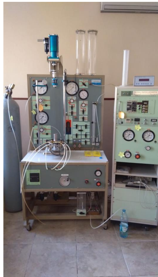
Figure 1. Cyclic triaxial device used in study
