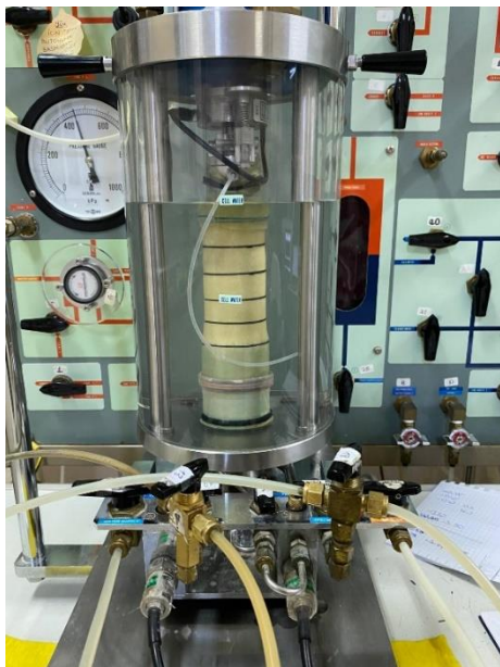
Figure 2. Consolidated specimen inside the cell before the loading stage.
