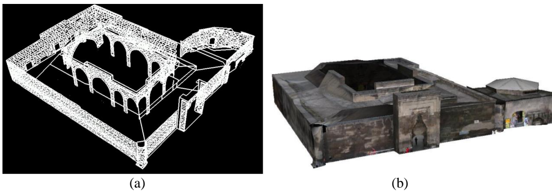
Figure 10. Kayseri Sahabiye Madrasah (a) 3D Scanning and (b) Model Created from Scanning [35]
