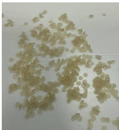
Figure 2. Sodium alginate microcapsule beads
