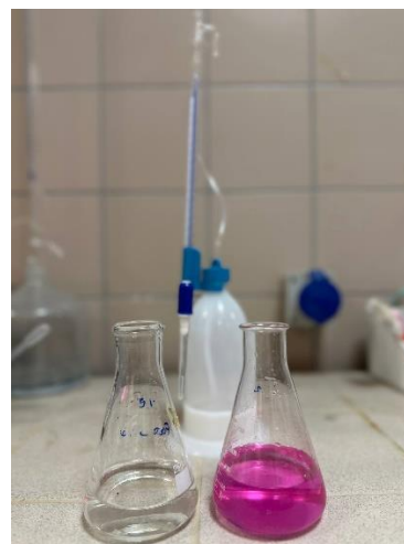
Figure 1. Titrator used for the titration process in the study, solution prepared for boron determination (left), titrated boron solution (right).
