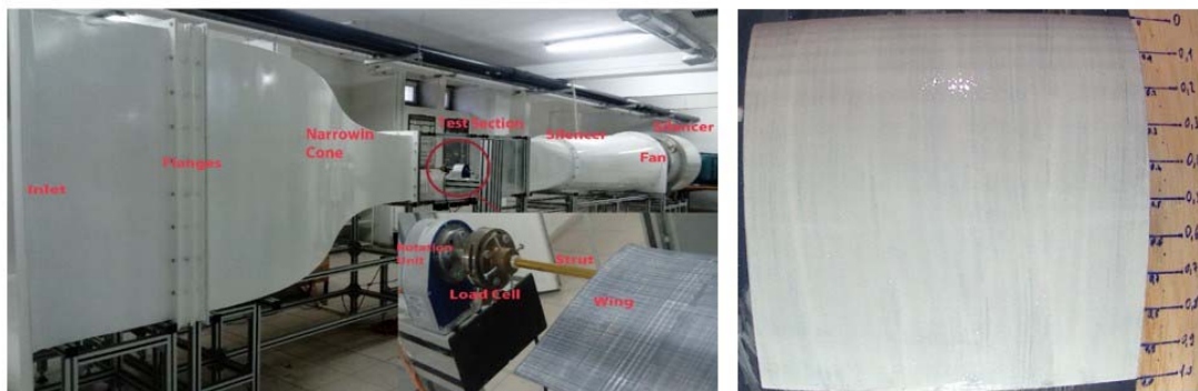
Figure 3. Views of the wind tunnel [25] and of the oil mixture on airfoil D surface
