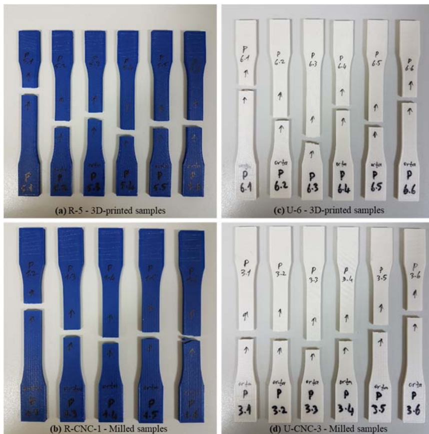
Figure 5. Images of broken samples
