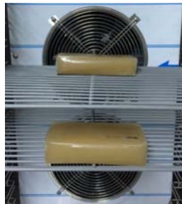
Figure 2. Placing the packages into the blast freezer
