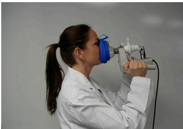
Figure 1: The correct way to hold the PAS external module during data capture (picture taken from PAS instructional manual)
