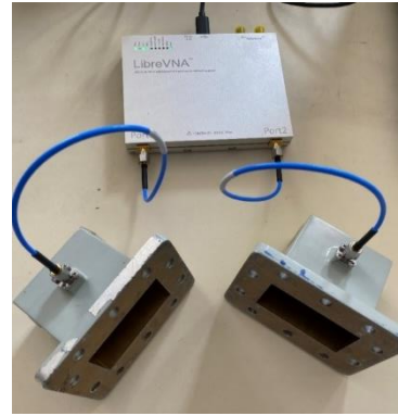
Figure 3. Shielding performance measurement mechanism.
