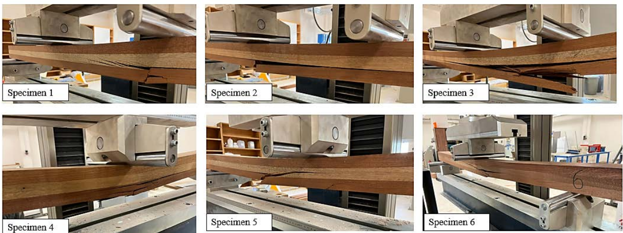
Figure 6. Failure modes of specimens.
