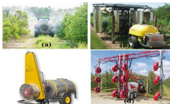
Figure 4. (a) VAA Fruit Orchard Sprayer (b) Tunnel Sprayer (c) Tower Sprayer (d) Multi-Channel Airblast Sprayer (Jadav et al., 2019).
