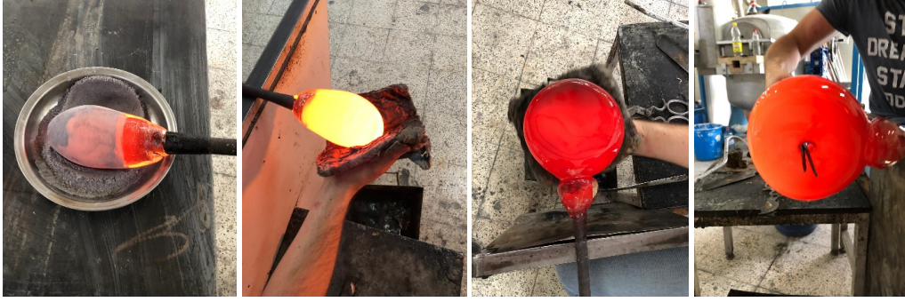
Figure 5. Powder color coating and forming process.
