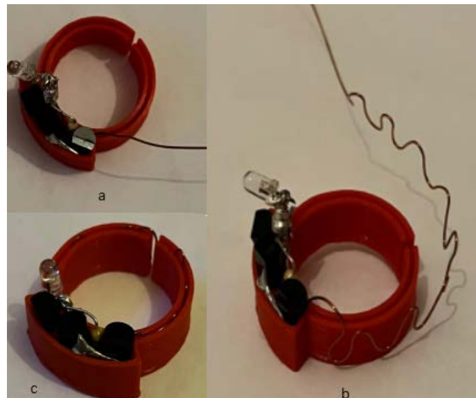
Figure 16. a) Placement of the sensing circuit in the design, b) Shaping the circuit antenna, c) Placement of the circuit antenna in the ring
