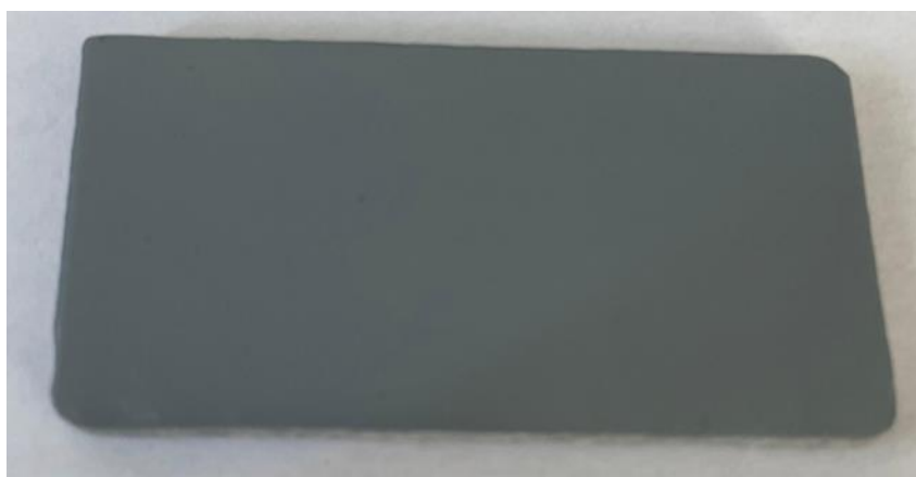
Figure 2. Paint Sample Containing \text{CoFe}_2\text{O}_4 Particles and Wood Shavings.
