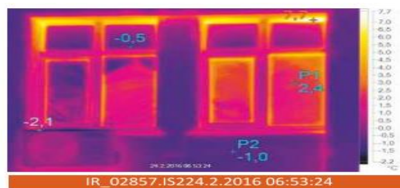
Figure1. Heat Loss through Window Openings [11].
