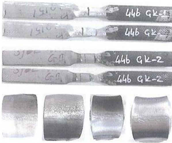
Figure 6. Tensile and 180° three point bending tested samples
