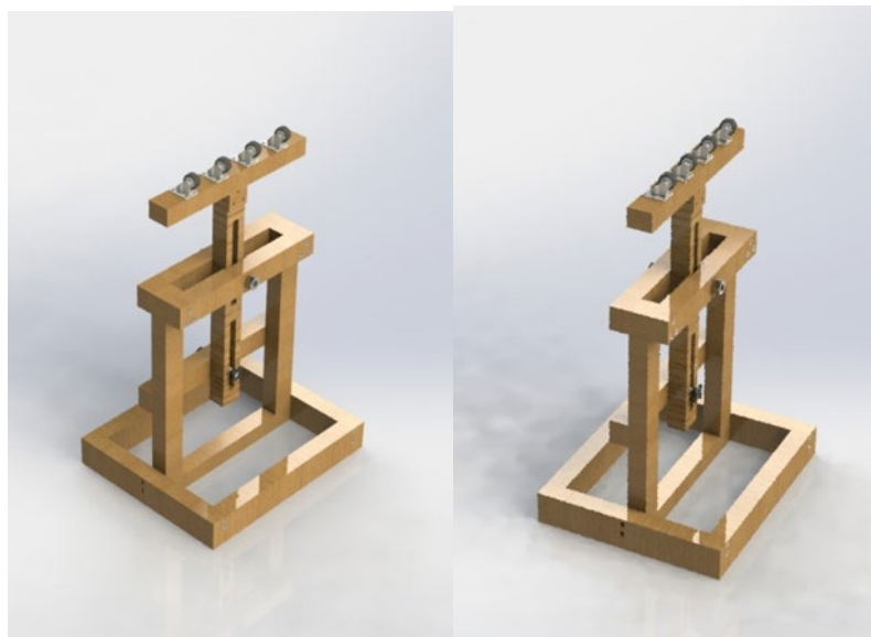
Figure 1: Pictorial view of the designed extension stand
