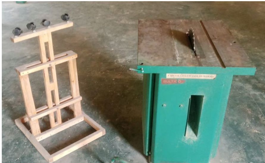
Figure 6. Extension stand ready for use with the table saw machine
