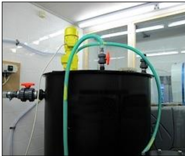
Photo 5. The bread digester for renewable energy (Biogas) in the Netherlands. Source: Enki Energy, by Stefan Blankenburg, 2016.
