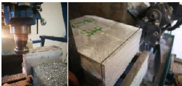
Figure 2. The chip removal process and cutting of the composites
