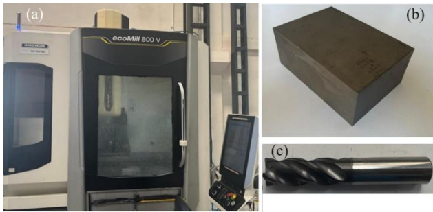
Figure 1. (a) EcoMill 800V 3-axis CNC machine (b) stock used in experiments (c) cutting tool used in experiments
