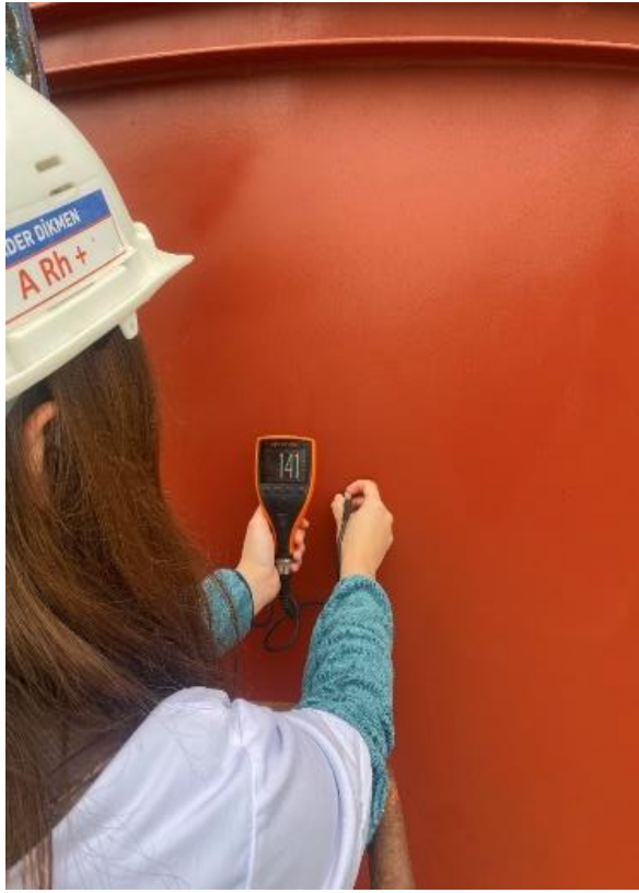
Figure 10. Measurement of primer paint thickness of silos
