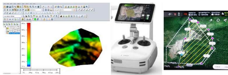
Figure 4. Creation of DEM data and preparation of flight plan
