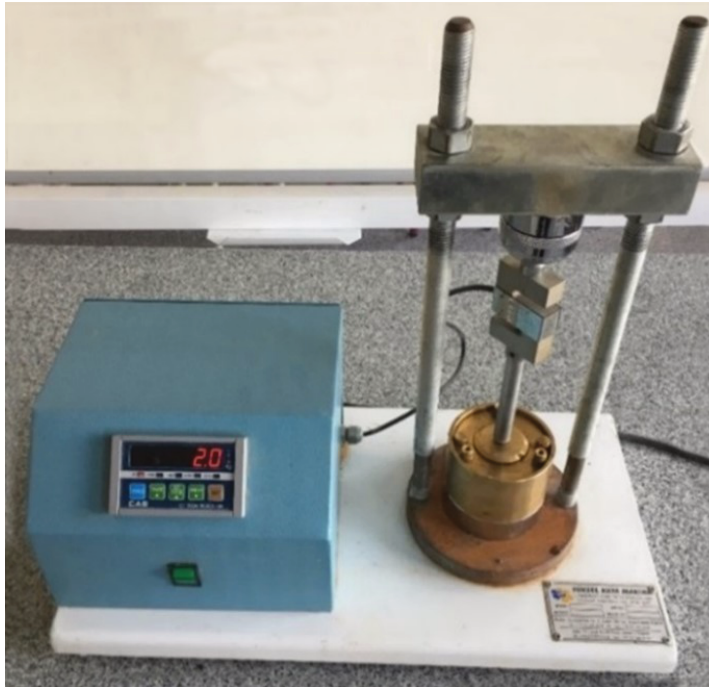
Figure 2- Swelling pressure test apparatus (from Kayabali and Yıldız, 2014).
