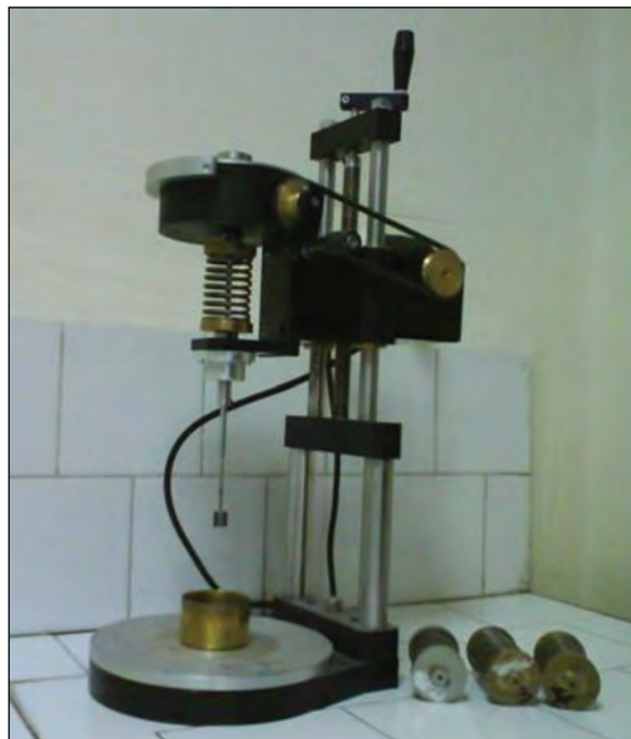
Figure 5- The old-fashioned vane shear test apparatus used in the earlier investigations of the lead author and his research group.
