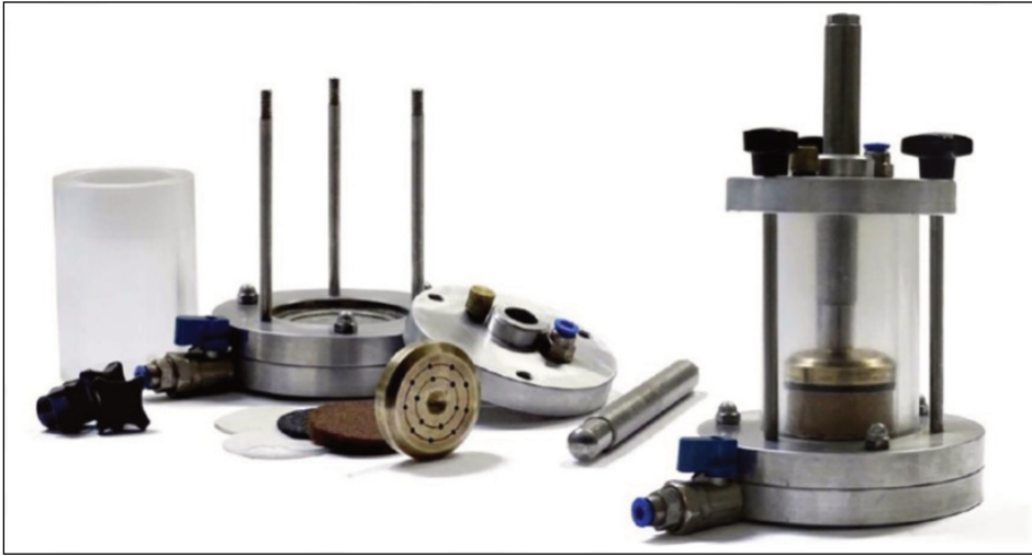
Figure 1- Permeability-consolidation test apparatus and its accessories (from Asadi, 2017).
