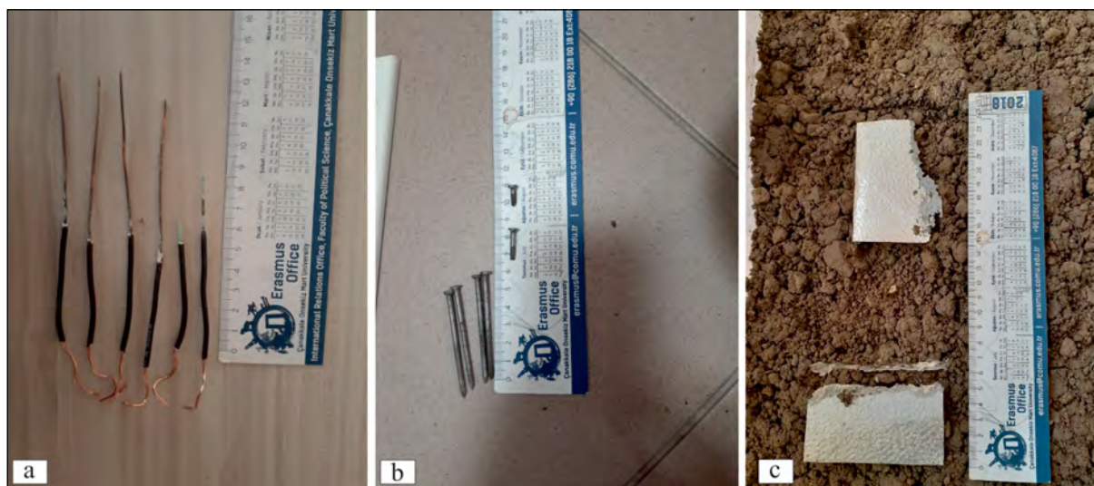
Figure 7- a) Corroded copper electrodes, b) Corroded galvanized steel electrodes, c) Corroded aluminum plate electrodes.
