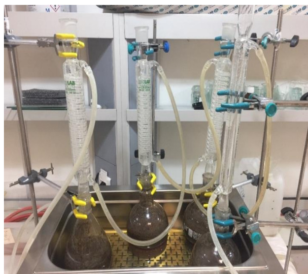
Figure 1. Water bath extraction at 60°C
